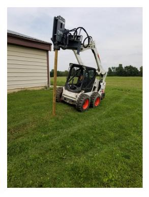
It's especially important to get a post driver that can swivel and still drive posts straight and true on hilly ground.
